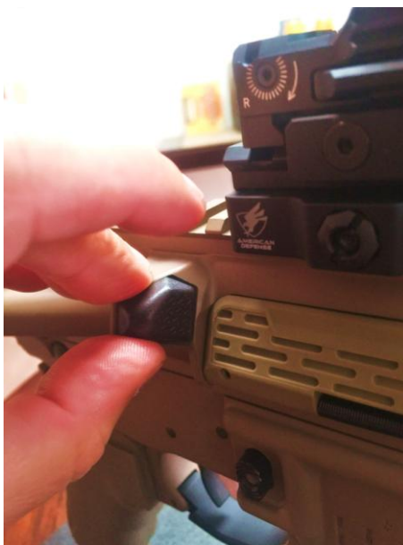
Step 2: Line the Deflector Brake up on the brass deflector as far forward as possible while ensuring the dust cover operates.
