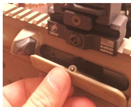
Step 2: Line the Deflector Brake up on the brass deflector as far forward as possible while ensuring the dust cover operates.
